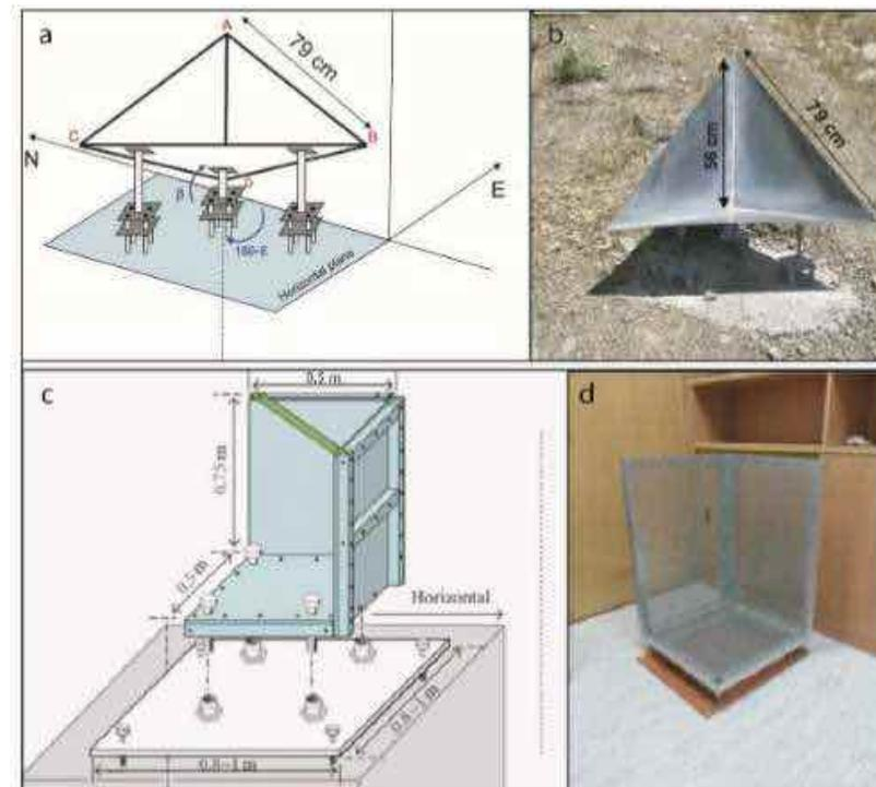
Corners reflectors (modified from Bovenga et al., 2017; and Qin et al., 2013)
