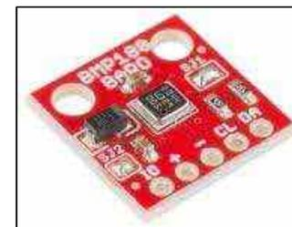
SparkFun **BMP 180 Barometric Pressure Sensor**
