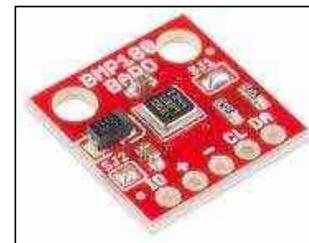
SparkFun **BMP 180 Barometric Pressure Sensor**
