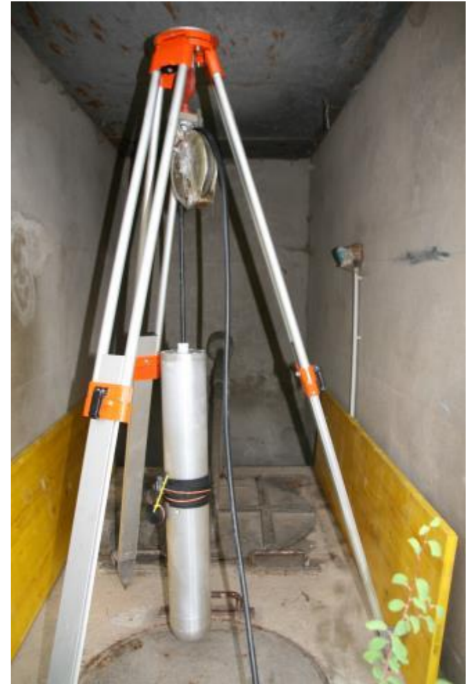
Testing one of the downhole tools
