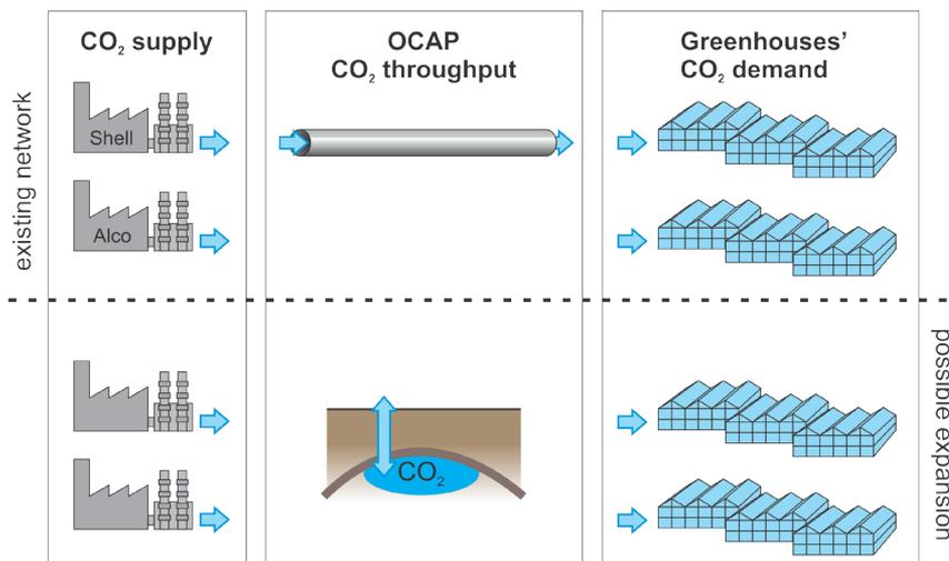
Figure 4: The existing network includes two CO<sub>2</sub> suppliers in the Rotterdam harbour area that deliver CO<sub>2</sub> to a pipeline, which transports it to several areas to be used in greenhouses (top). The lower illustration shows potential elements for expanding the network, such as additional suppliers and consumers, but the current bottleneck is the buffering capacity of the network.
