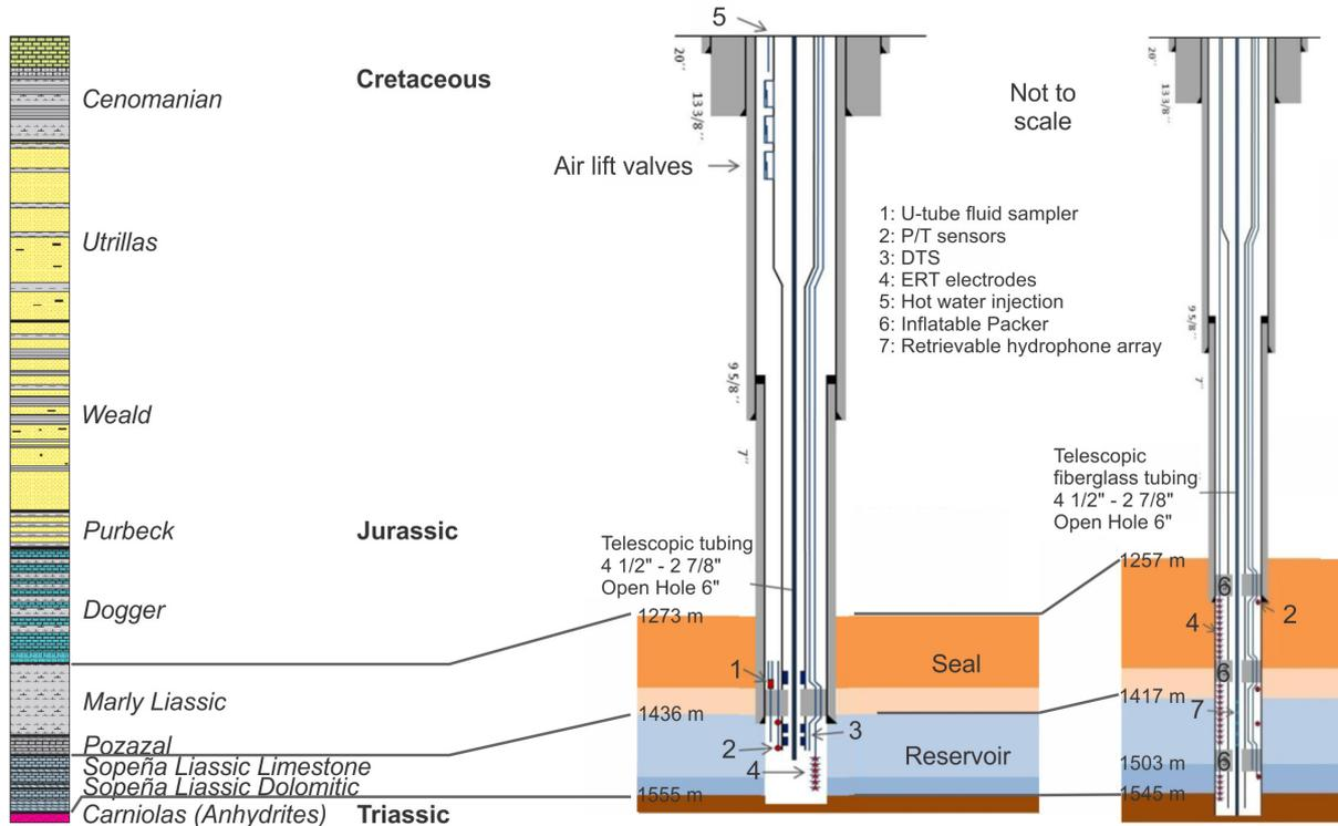
Figure 1: Lithological column on left side describes geological formations of the seal and reservoir. Injection well (middle) and observation well (right) with their deep monitoring devices form part of the Hontomín TDP.
