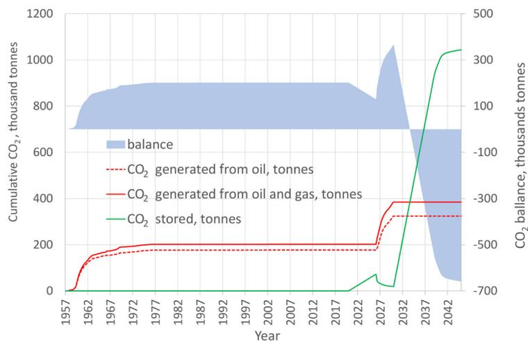
Figure 3: CO<sub>2</sub> balance of one of the initial simulations for the LBr-1 field. On the horizontal (time) axis we can identify the historical phase of conventional oil production, the long relaxation period after site abandonment, and the potential future CO<sub>2</sub>-EOR and CO<sub>2</sub> storage phases.
