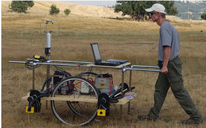
Open path IR lasers (CO<sub>2</sub> and CH<sub>4</sub>) - BGS
