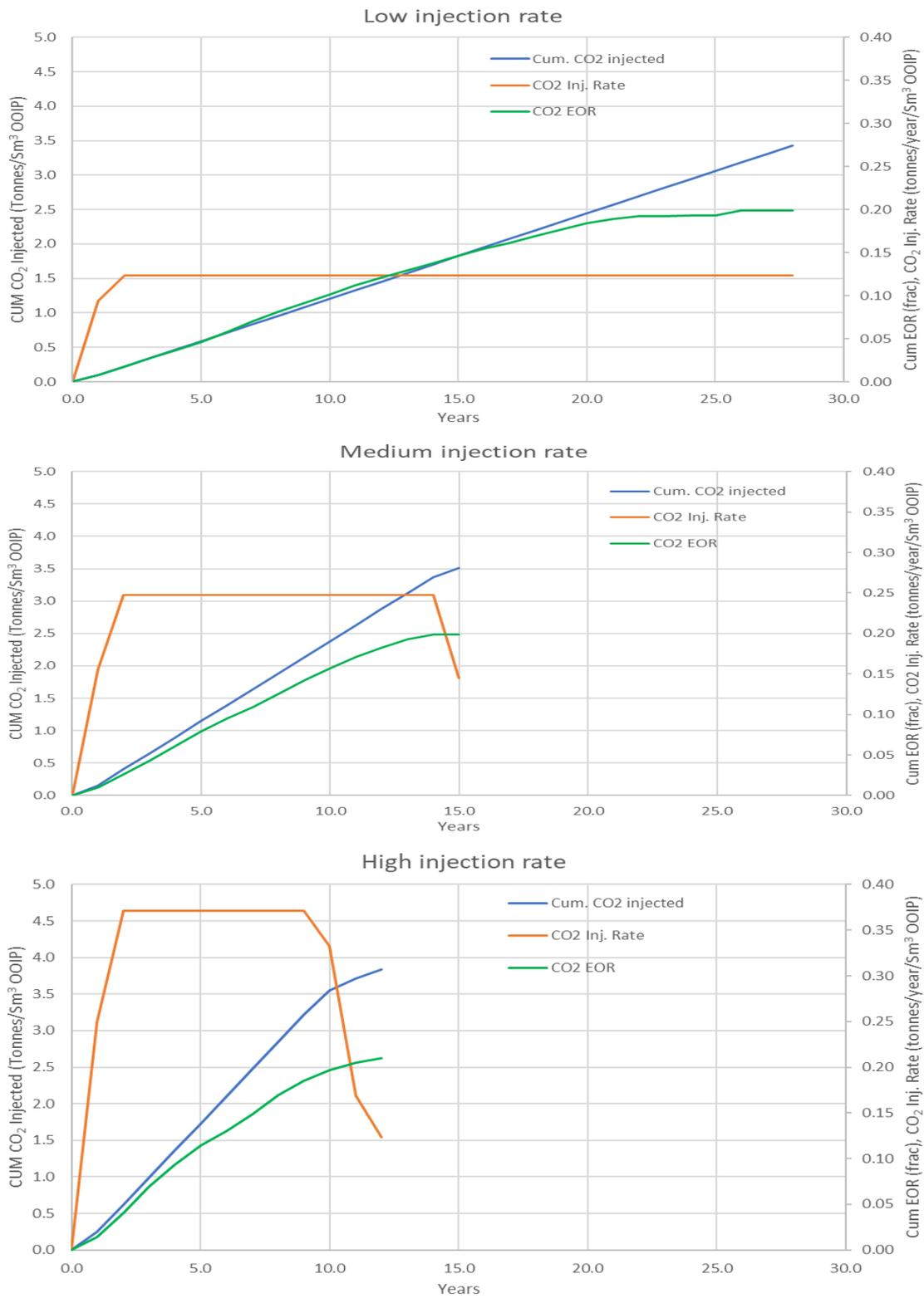
Figure 36. EOR efficiency vs CO<sub>2</sub> injection rate.
