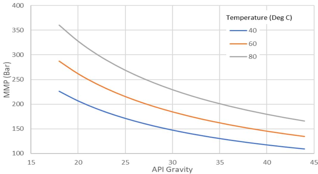
Figure 45. Minimum miscibility pressure for CO<sub>2</sub> in oil (reproduced from (Bachu, 2016)).
