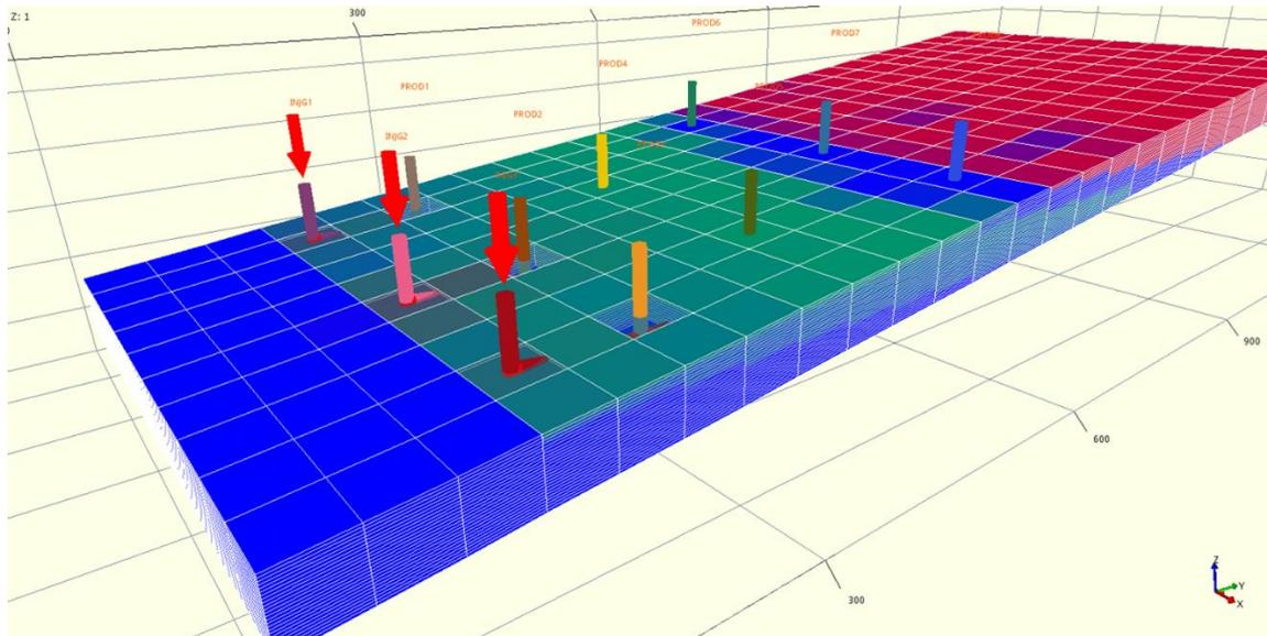
Figure 33. Reservoir model, prior to CO<sub>2</sub> injection.
