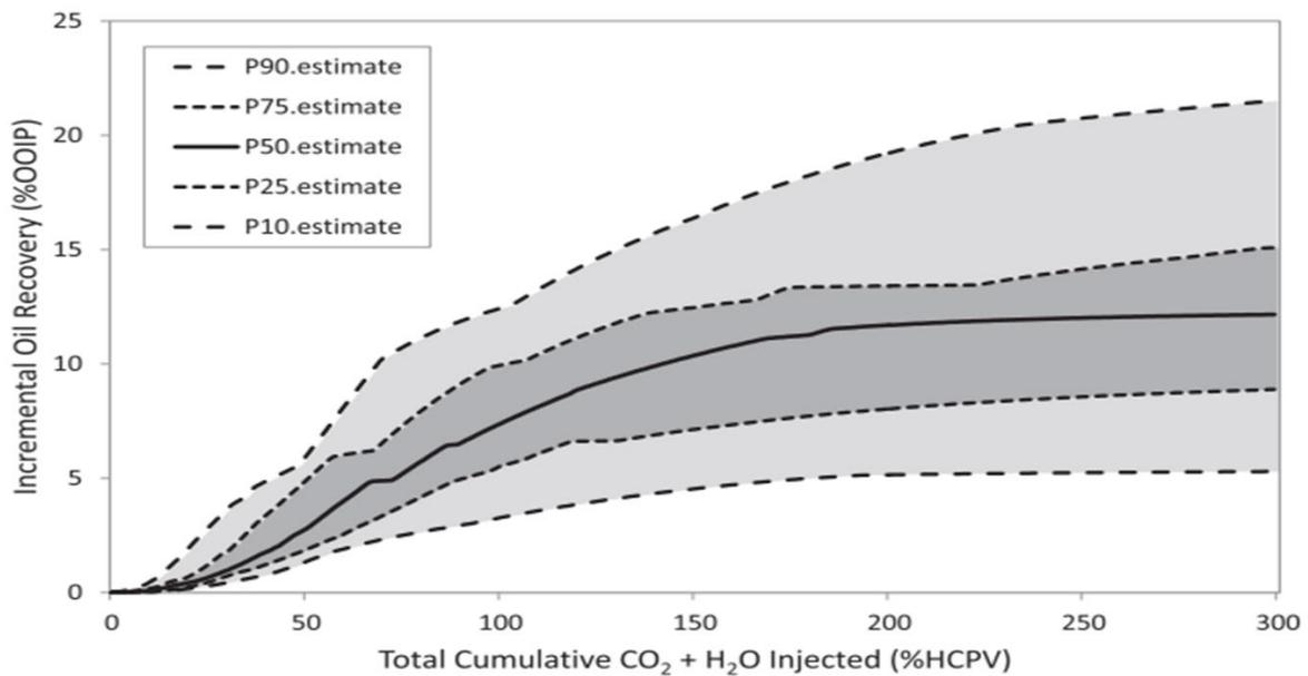
Figure 35. Incremental oil recovery from CO<sub>2</sub>-WAG flooding (exerted from Azzolina & et al. 2015).
