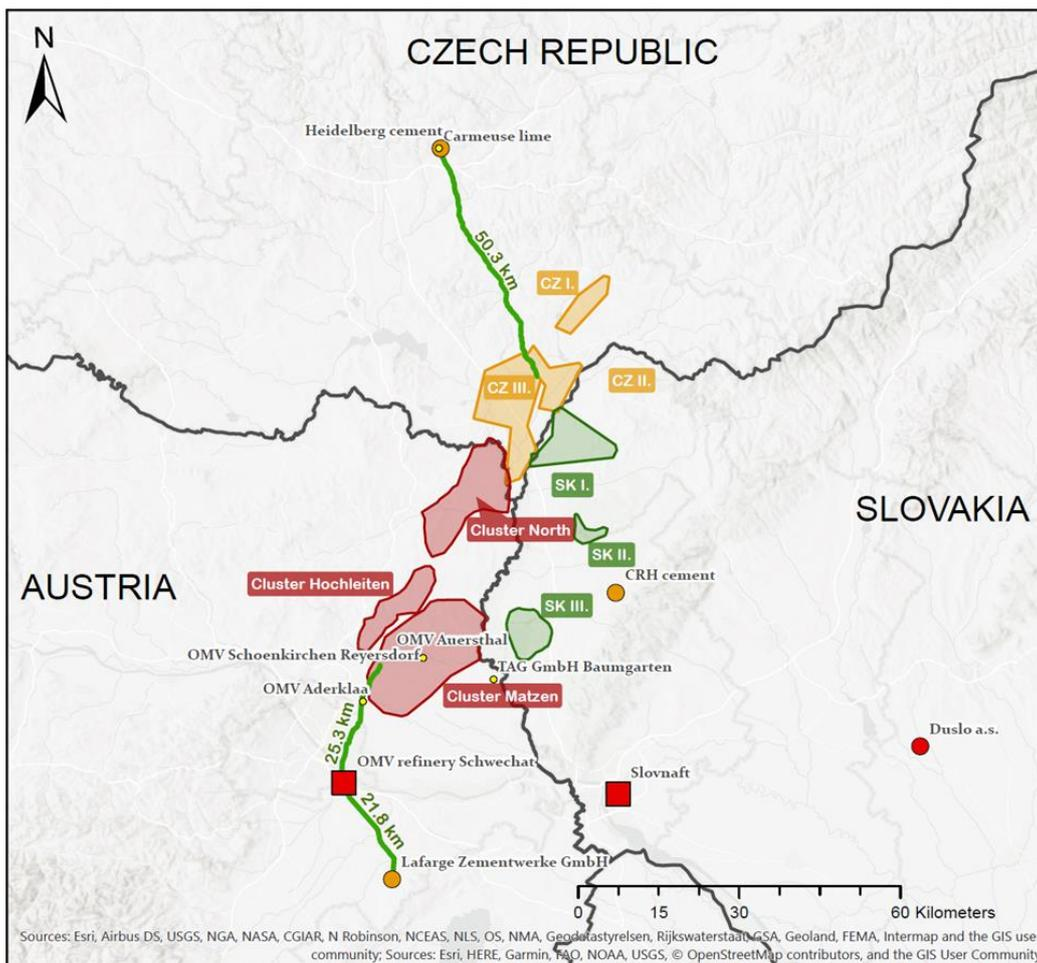
Figure 42. Results of source sink matching showing the locations of the selected sources (the Czech HeidelbergCement plant, the OMV refinery and the Lafarge cement plant in Austria), as well as the oil fields clusters. Green lines depict the calculated indicative pipelines based on considerations explained in Chapter 6.1. Note that pathways might differ for the case study No. 2 as existing pipeline networks were not evaluated in Chapter 6.1.
