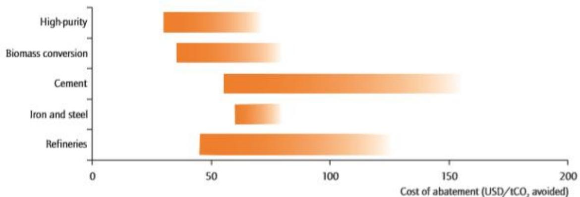
Figure 39. Ranges of estimated cost of CO<sub>2</sub> capture from different industrial processes. 'High purity' includes natural gas processing, hydrogen production and ethylene oxide production (IEA 2011).
