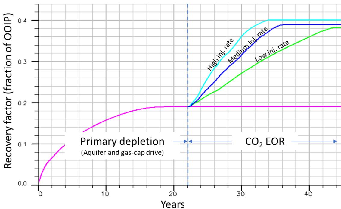
Figure 34. Example recovery profiles exhibited by the concept models.
