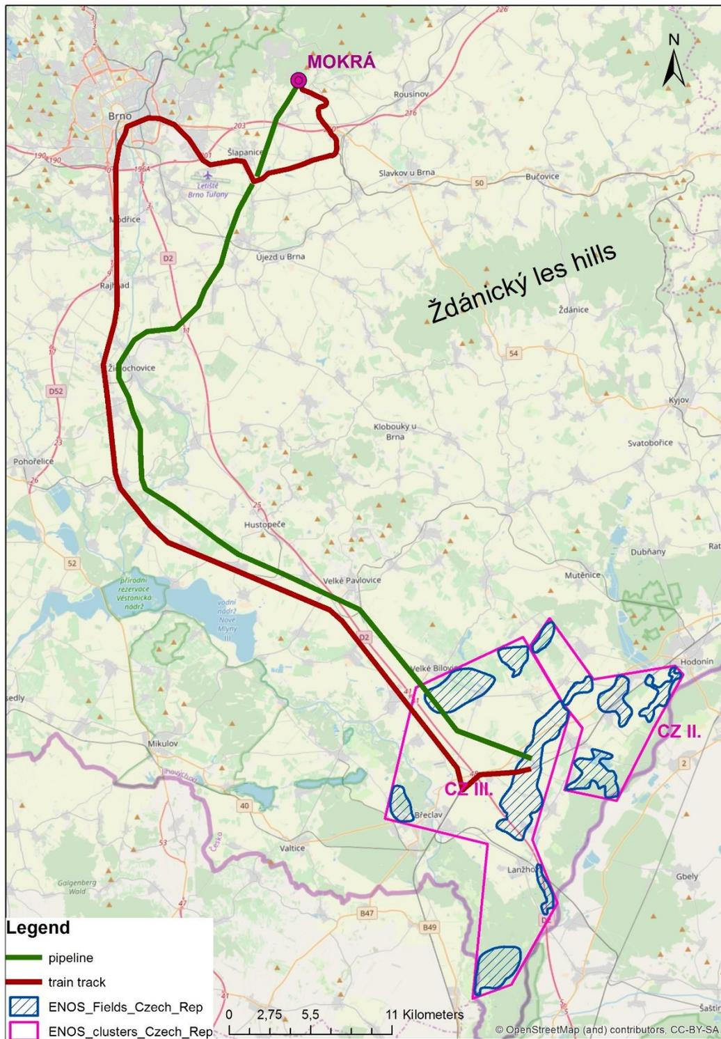
Figure 44. Possible CO<sub>2</sub> transport routes between the Mokrý cement plant and cluster CZ III.
