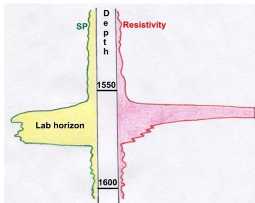
Figure 16. Example of SP and RAG well logs showing typical properties of the Láb horizon – low SP values and high resistivity.
